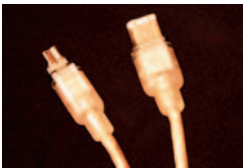
Small and Large Firewire Connectors
